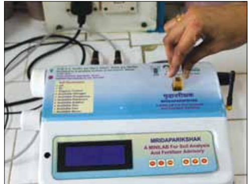
Mridaparikshak: A minilab for soil health assessment and fertiliser advisory
