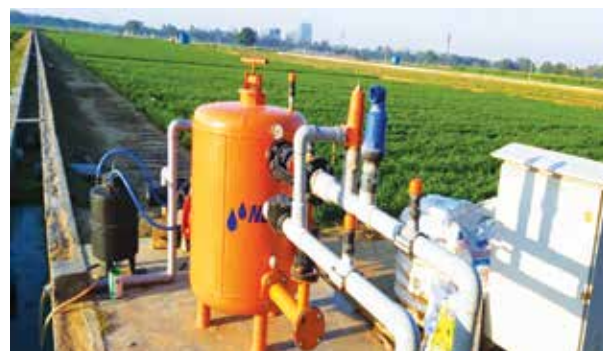
Sub-surface drip fertigation system in maize-wheat system
