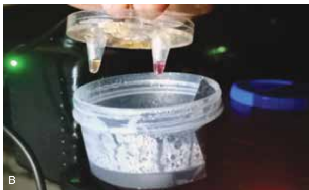
A) The device is connected to the power source. B) The colorimetric assay was executed with the help of the designed device for LAMP-based detection of pathogens. Yellow colour marks the presence of Rhizoctonia solani AG 1 IA in rice sheath, whereas pink colour denotes no template control.
