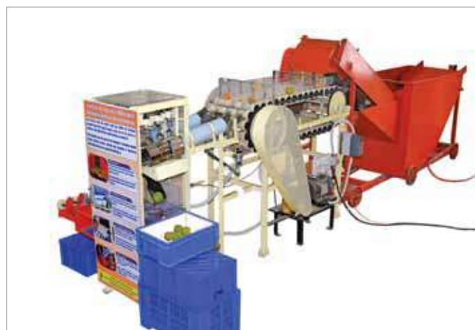
Automated packaging line for spherical horticultural crops
