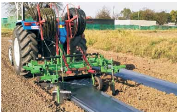
Tractor operated drip lateral-cum-plastic mulch laying machine
