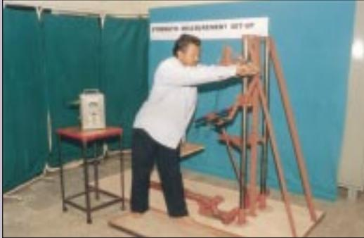
A strength measurement set-up for agricultural workers. Strength data of male as well as female agricultural workers have been collected to test working of the strength measuring set-up and to chalk-out protocol.
