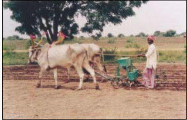
CIAE planter. Animal-drawn this machinery saves 64% on the operation cost compared to conventional method of sowing behind the country-plough with manual seed-dropping.
