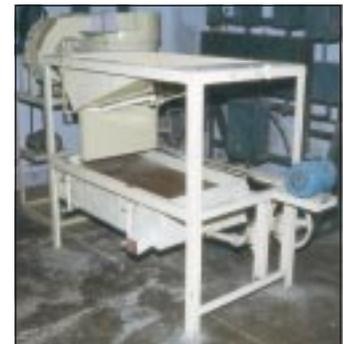
Cleaner for reducing dust emission in *dal* mill. A prototype of the cleaner equipped with suitable ducts, a forward curved centrifugal blower and a cyclone separator to arrest dust emission in *dal* mills has been developed. This is 68-87% screen effective unit, and purity of cleared grains is over 98%.
