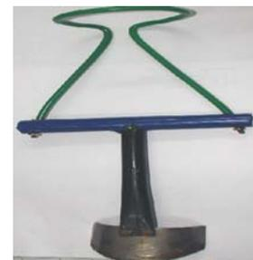
Banana-comb cutter facilitates cutting and separation of banana comb with minimum damage
