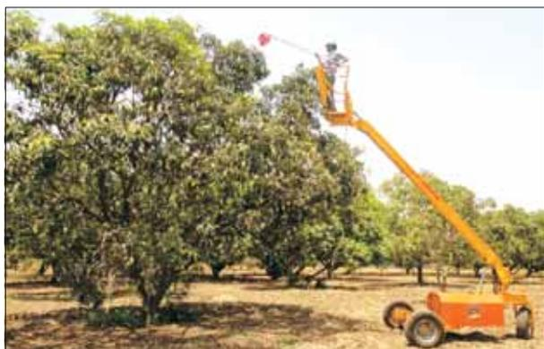
Self-propelled hydraulically hoisted platform for orchard management
