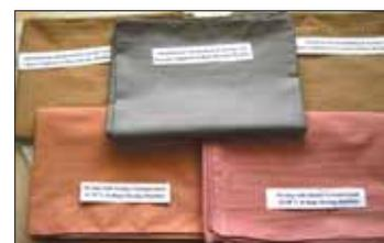
Samples dyed in rope-dyeing machine
