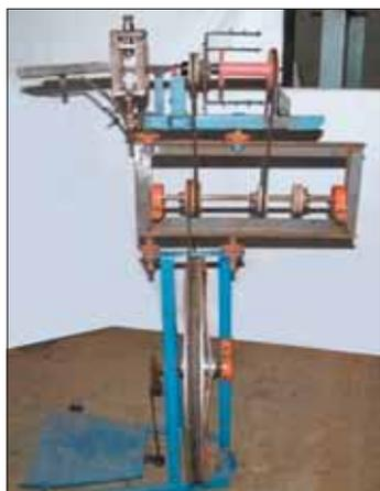
produce various types of yarns; their tensile characteristics were found at a par with mill-made yarn. With this *charkha*, a yarn count as fine as 149 tex (4s Ne) could be produced for making home - furnishing fabrics.
