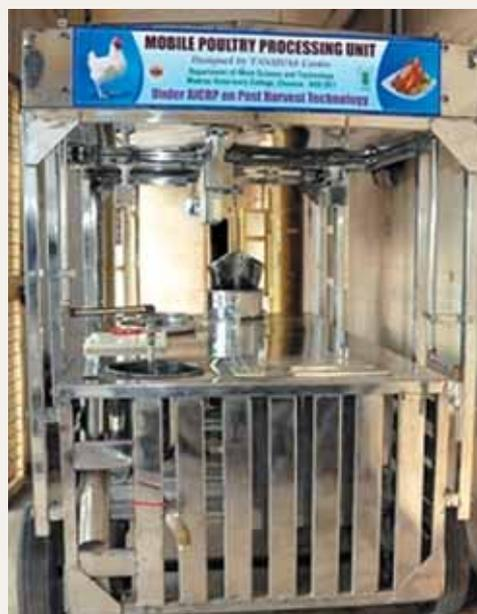
The stainless steel unit weighing 500 kg is of 2,410mm × 1,345mm × 2,058 mm, and costs approximately ₹ 5.50 lakh (2012-13). Its capacity is 35-40 birds per hour. It consists of two water tanks, bleeding cones and troughs, a scalding tank, a de-feathering machine, a carcass washing unit, a teflon board for cutting carcasses, an insulation box, crates for holding 50 line birds and work area for preparation of value-added products.
