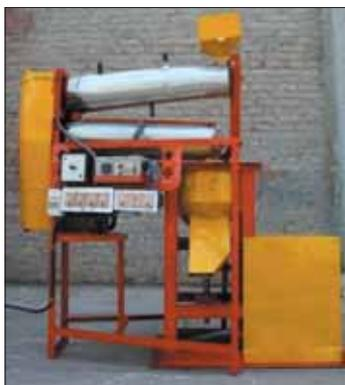
**Automatic custard-apple pulper:** The pulper performs three functions— fruit-cutting, fruit-scooping and pulping. Fruit-cutting part of the machine has two opposite rotating rollers with fruit-holding cups. Fruits are cut into two halves by a stainless-steel knife. The cut-halves are inverted and moved on to a stainless steel sieve and are pressed by a pressing plate. The seeds pass through the sieve, and peel remains on it.
