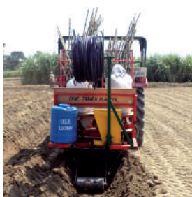
Sugarcane trench planter with attachments for laying of sub-surface drip laterals
