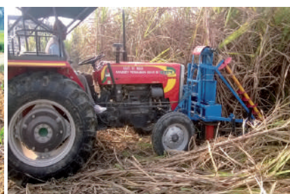
Sugarcane harvester for cutting of two rows of whole cane stalks and windrowing it linearly between tractor wheels
