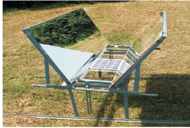
Concentrator for solar photovoltaic panel
