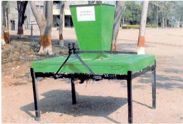
Tractor-mounted banana shredder
