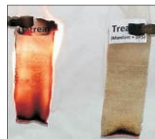
Fire retardant jute fabric using natural extract
