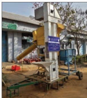
Motorized protray, poly bag and pot filling machine for horticultural nursery
