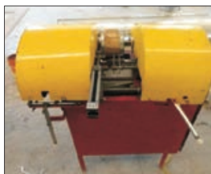
Composite peeler-cum-juice extractor for sweet orange and kinnow
