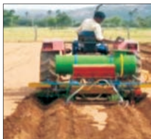
Tractor operated variable width raised bed planter
