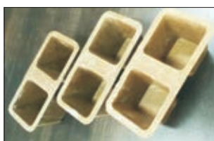
Seedling tray from nano-lignocellulosic biomass based composites
