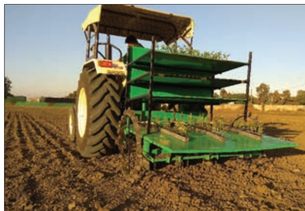
Tractor operated automatic vegetable transplanter for plug type seedlings
