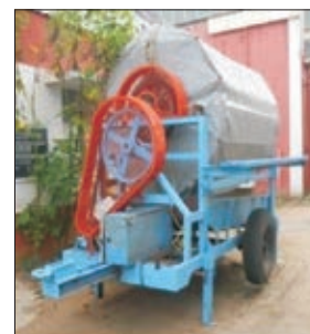
Turmeric polisher for dust reduction
