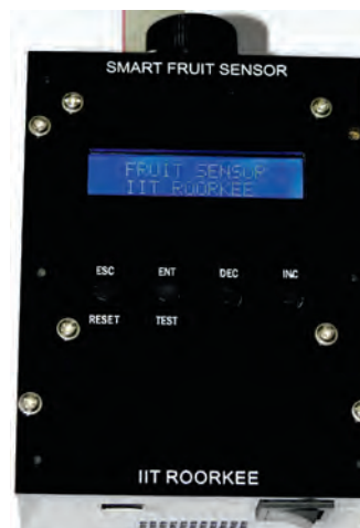
Fruit-nose sensor prototype to measure apple ripeness
