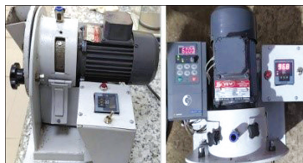
Pearl millet decorticator developed having different degree of decortication from 2–20%
