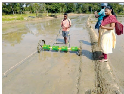
Direct Seeding of Rice with drum seeder (KVK, Chittoor, Andhra Pradesh)
