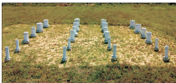
Mini pan evaporimeters (GI and PVC) of different sizes installed at IIWM
