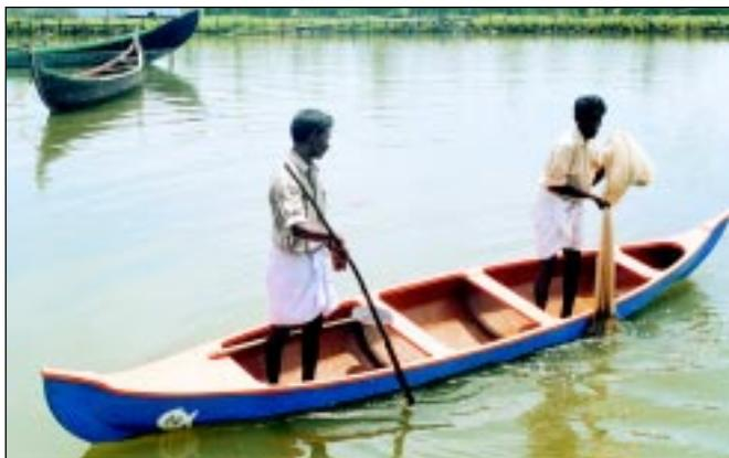
Canoe constructed from rubber wood
