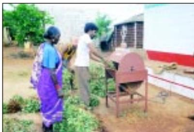
Groundnut stripper was developed at the CRIDA, Hyderabad. Its efficiency is maximum at 400 rpm for 1-day-old harvest
