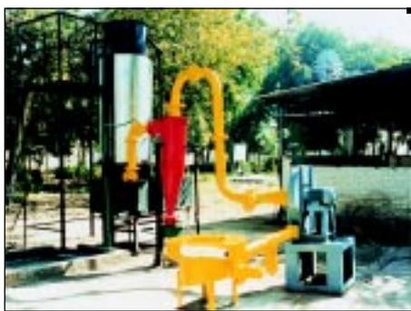
**Groundnut-shells-based Open-core Gasifier.** The fuel used for the system is dry groundnut-shells and groundnut-shell briquettes. In the system, every 4 kg of groundnut-shells replaced 1 litre of light diesel oil
