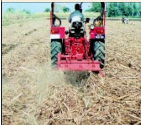
**Tractor-mounted sugarcane trash-shedder.** Its soil-mixing blades dig soil from the sides of the ridges and mix it with chopped trash. Due to its soil digging, fibrous roots of stubbles could be removed; which is useful for the ratoon-crop
