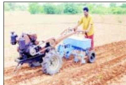
Power tiller-drawn seed-cum-fertilizer drill/planter was engineered for sowing blackgram, greengram, sorghum, groundnut, maize and castor. It has an area coverage of 0.25–0.3 ha/hour
