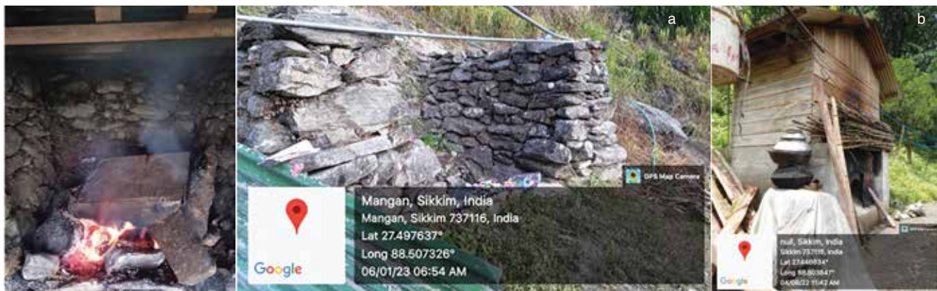
Combustion drying of large cardamom in (a) Traditional and (b) Improved bhattis at Dzongu, north Sikkim
