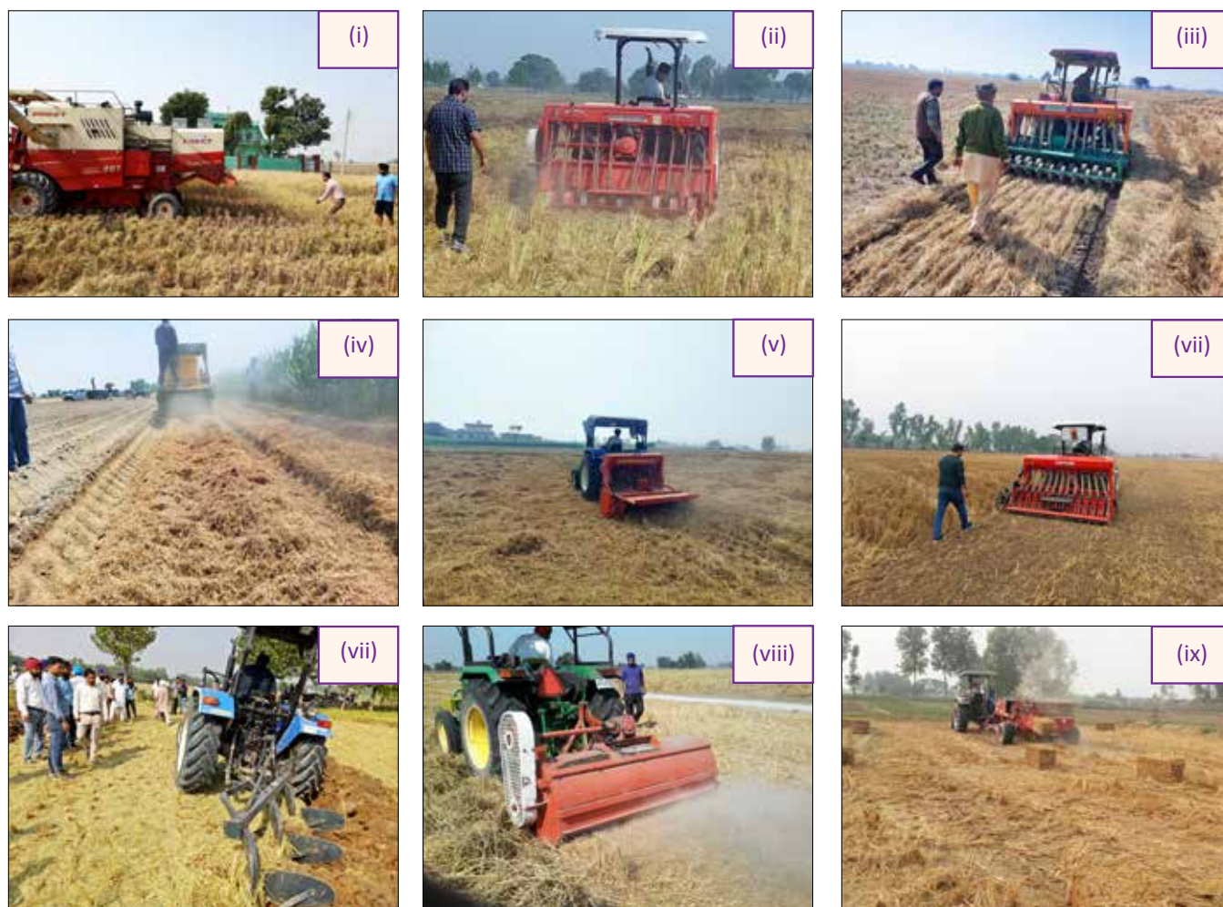
Farm machinery involved in paddy residue management; (i) PPA Super SMS attached combine harvester; (ii) Happy Seeder; (iii) PPA Smart Seeder; (iv) Paddy Straw Bale Shredder-cum-Mulcher; (v) PPA Surface Seeder; (vi) Super Seeder; (vii) Mouldboard plough; (viii) Paddy straw chopper; (ix) Baler
