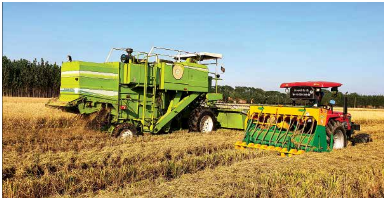
Combo technology of super SMS fitted combine and sowing of wheat with Happy Seeder
