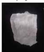
Banana cellulose acetate-based electrospun film
