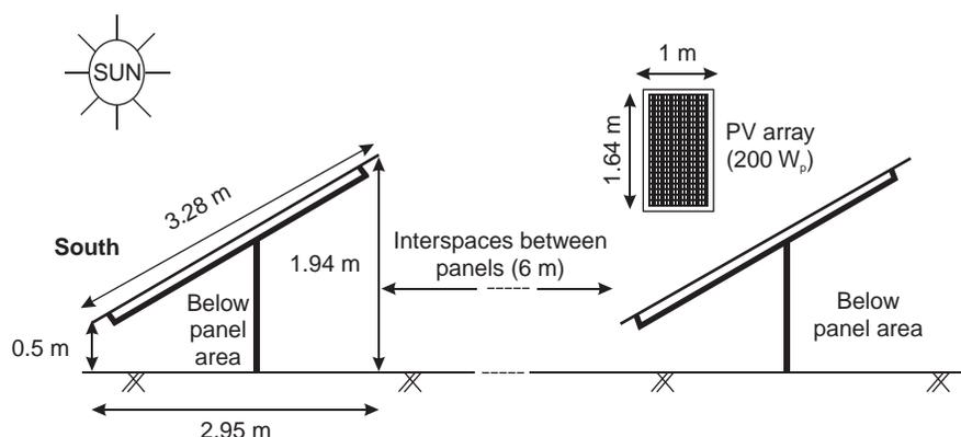
Fig. 2. Design of typical agri-voltaic system.
