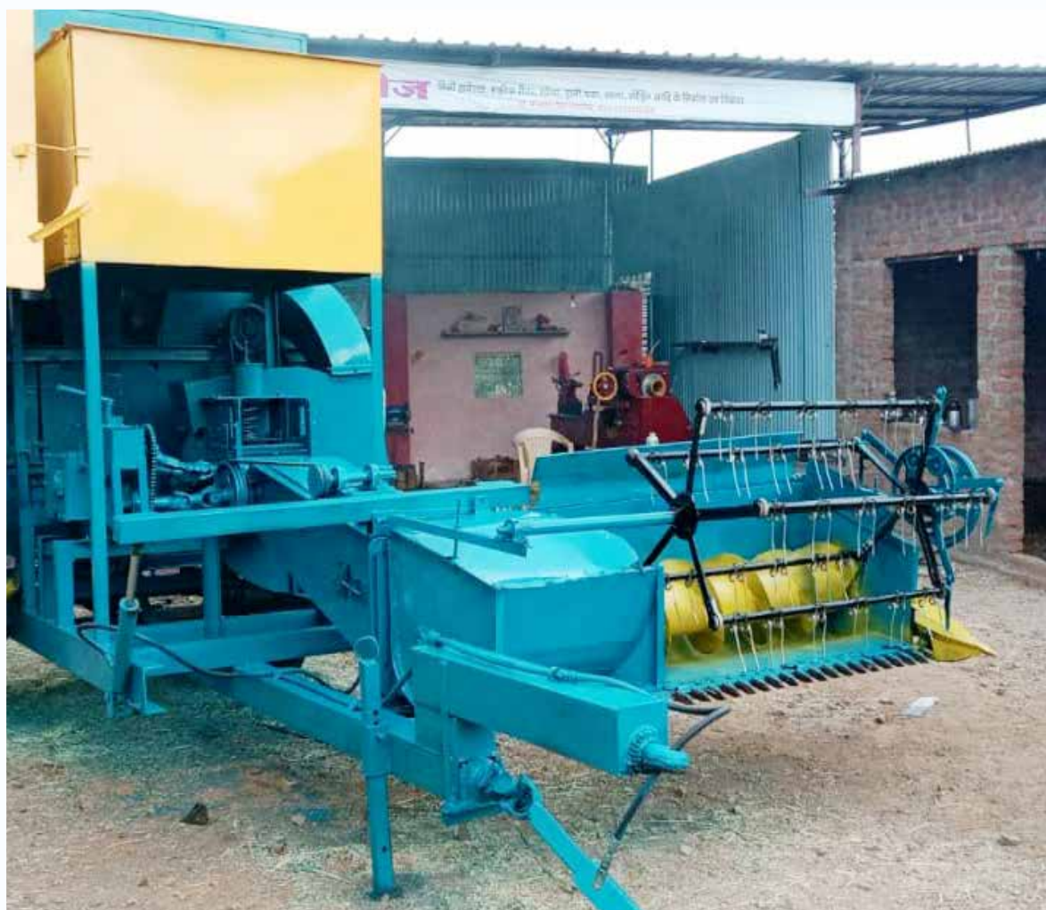
View of combine harvester with straw collection mechanism
