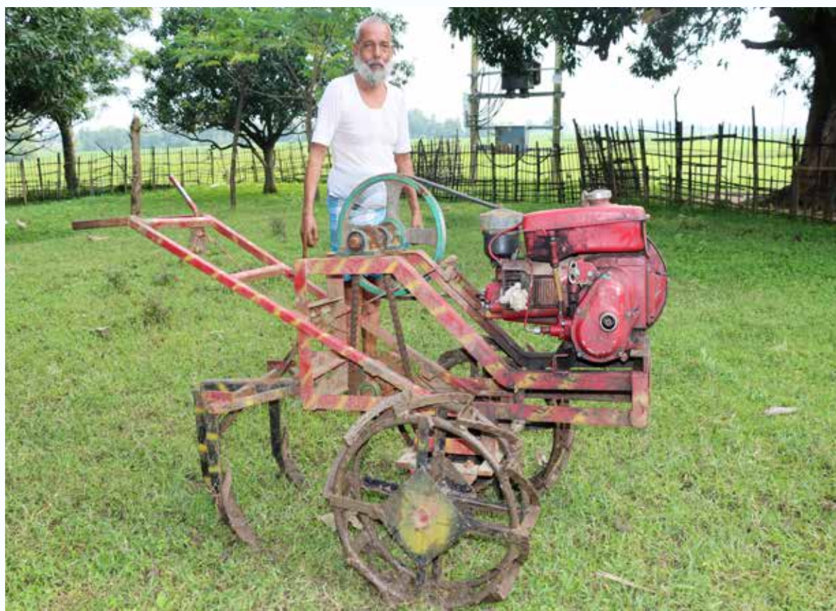
Low-cost power-tiller-cum-zero tillage machine
