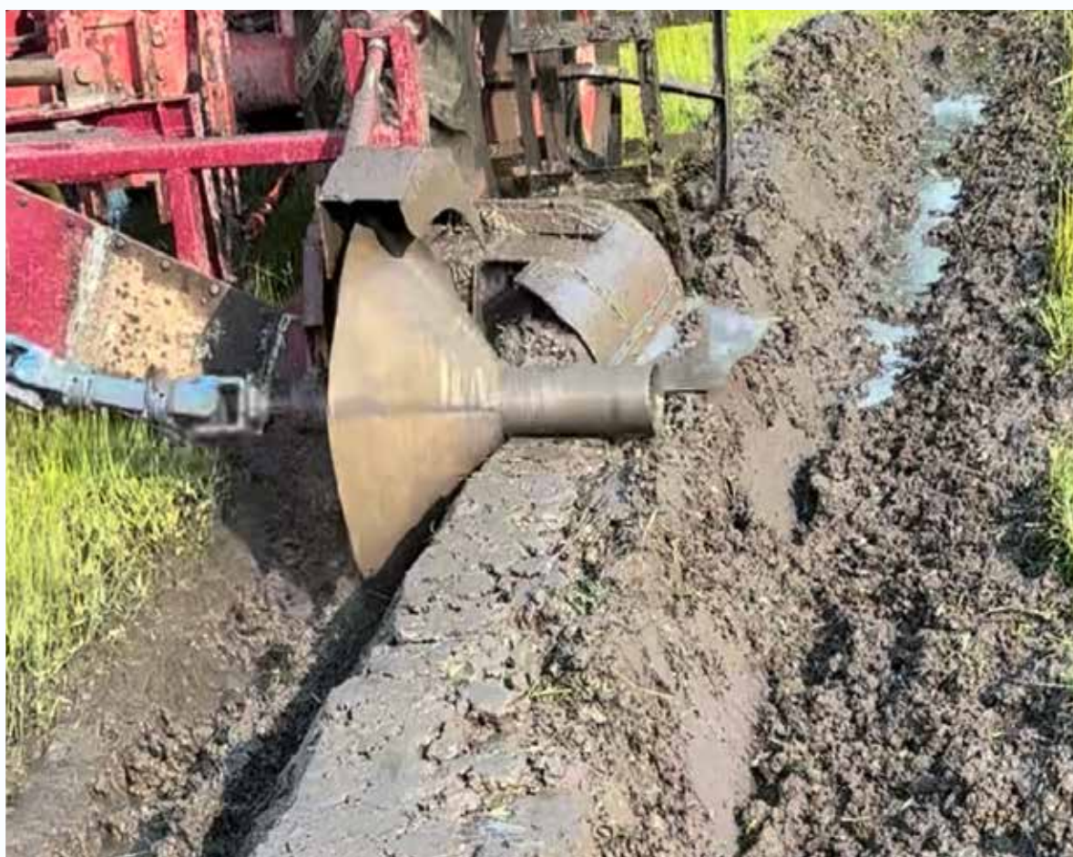
Tractor-mounted bund maker in action
