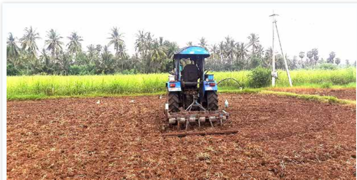
View of cultivator cum drum seeder in the field
