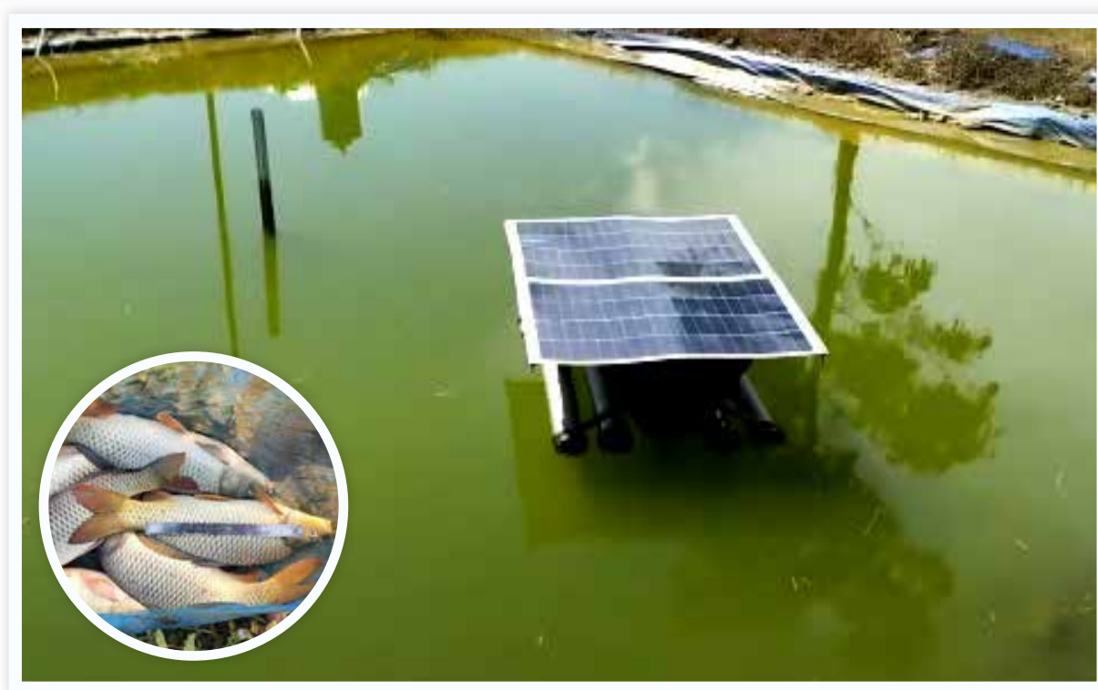
Solar powered feed dispenser-cum-aerator floating in pond
