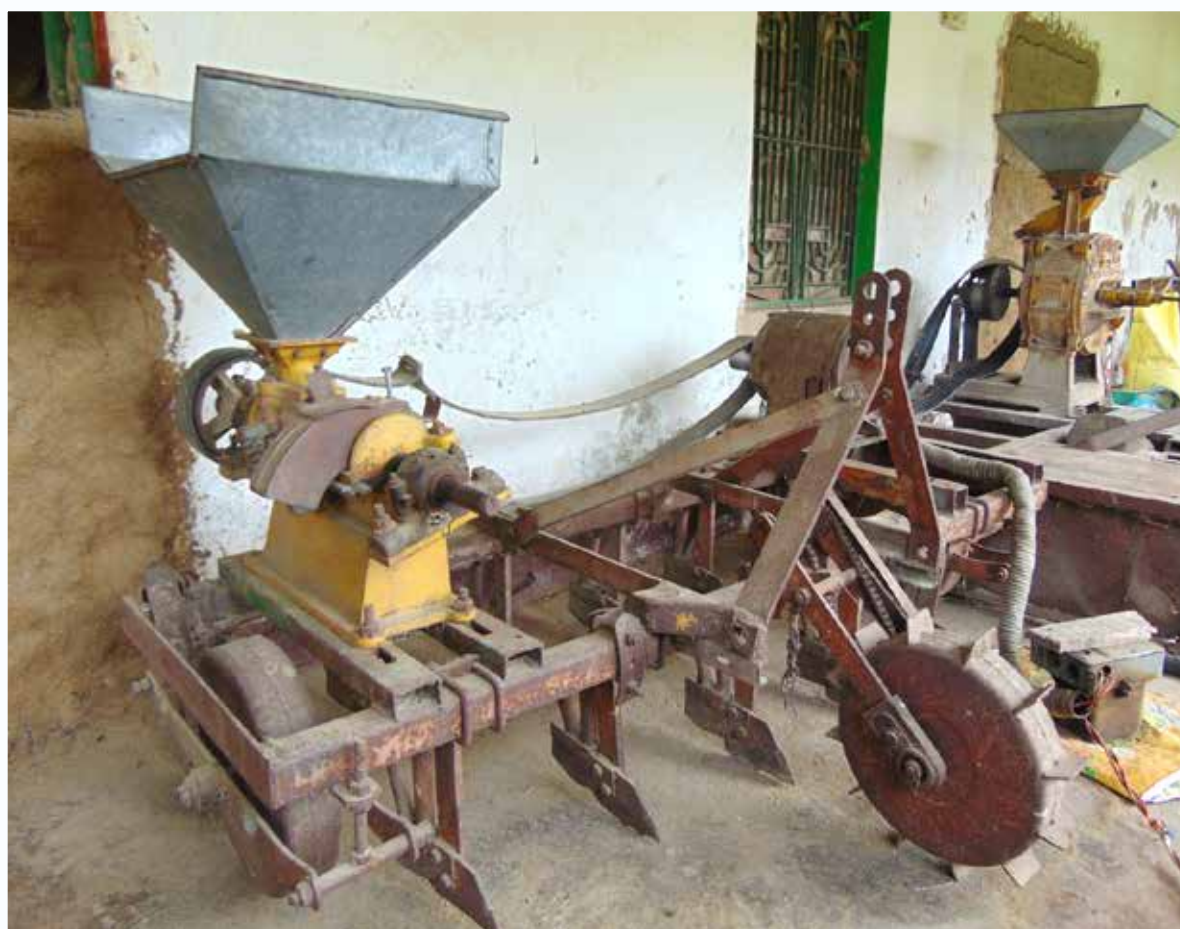
Rice huller fixed on zero-till machine
