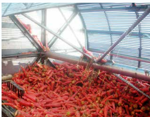
Inside view of a carrot washing machine
