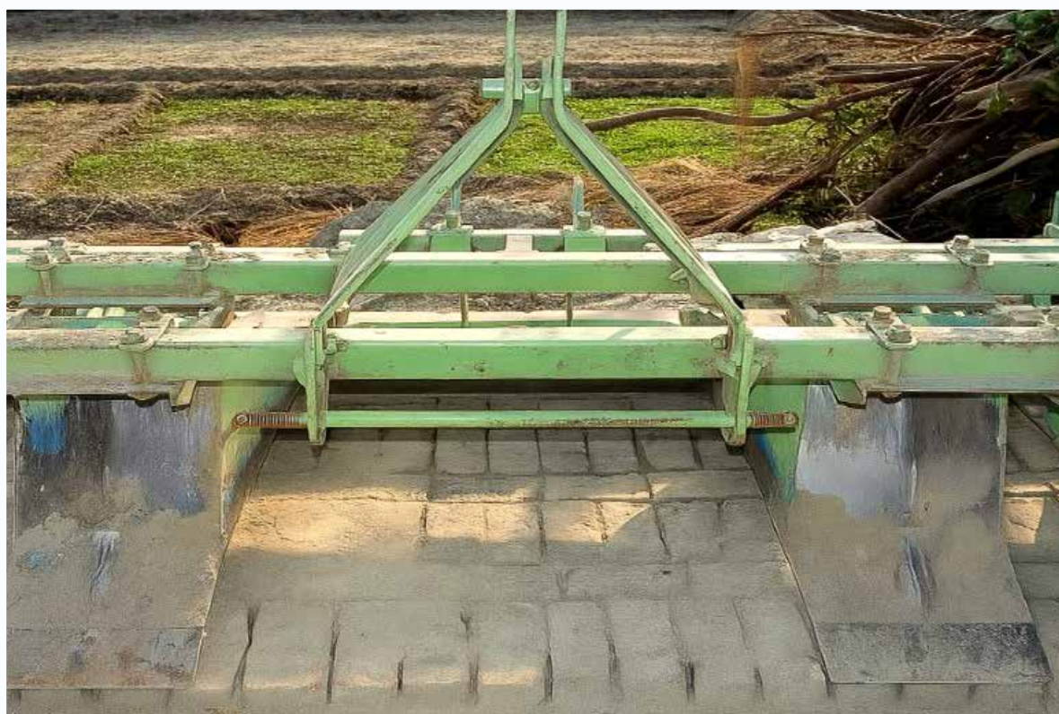
Modified sugarcane trench opener for mechanized irrigation
