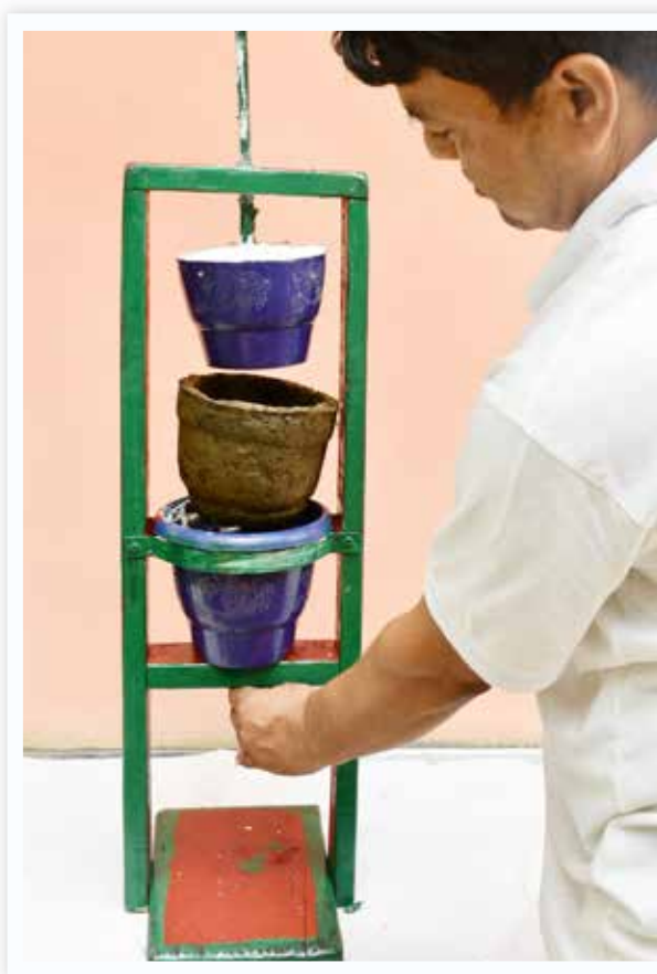
Cow dung pot preparation from Press Machine
