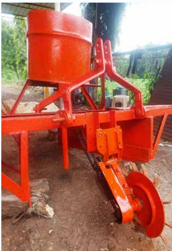
Ridge - bund maker with adjustable fertilizer application
