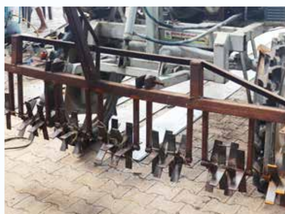
Custom built DSR machine fitted on jugad
