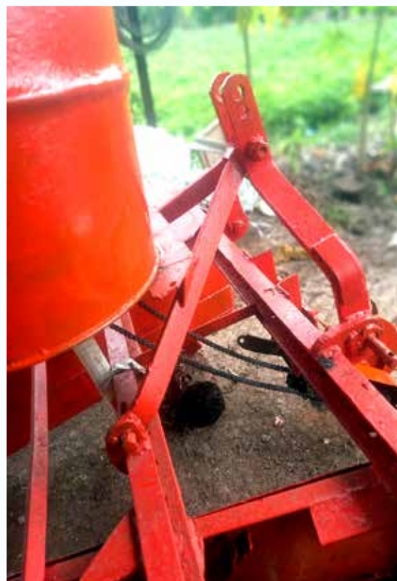
Ridge - bund maker with adjustable fertilizer application
