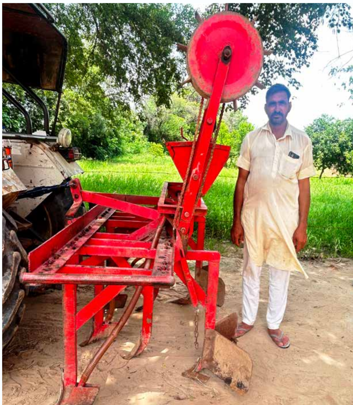
View of weeder cum fertilizer applicator
