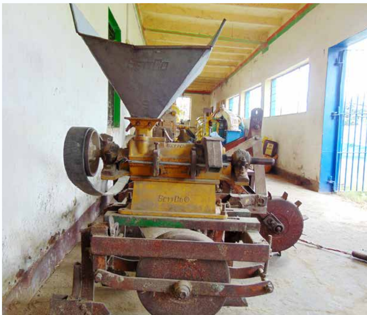
Machinery for grain cleaning fitted on zero-tillage machine
