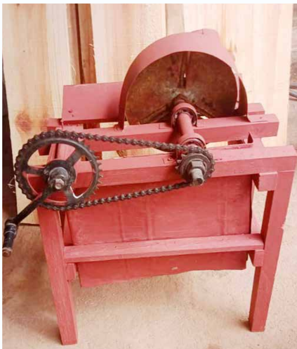
Close view of hand operated ginger cum turmeric slicer
