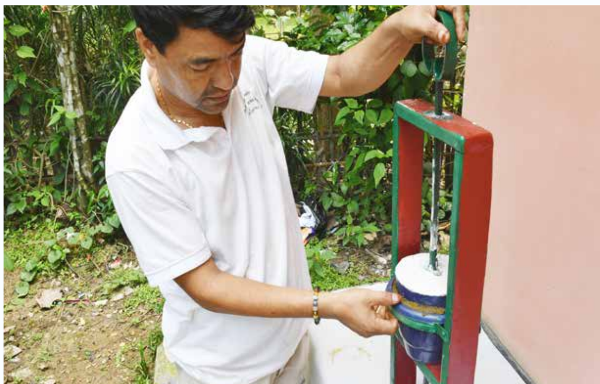
Press Machine for preparing cow dung nursery cup
