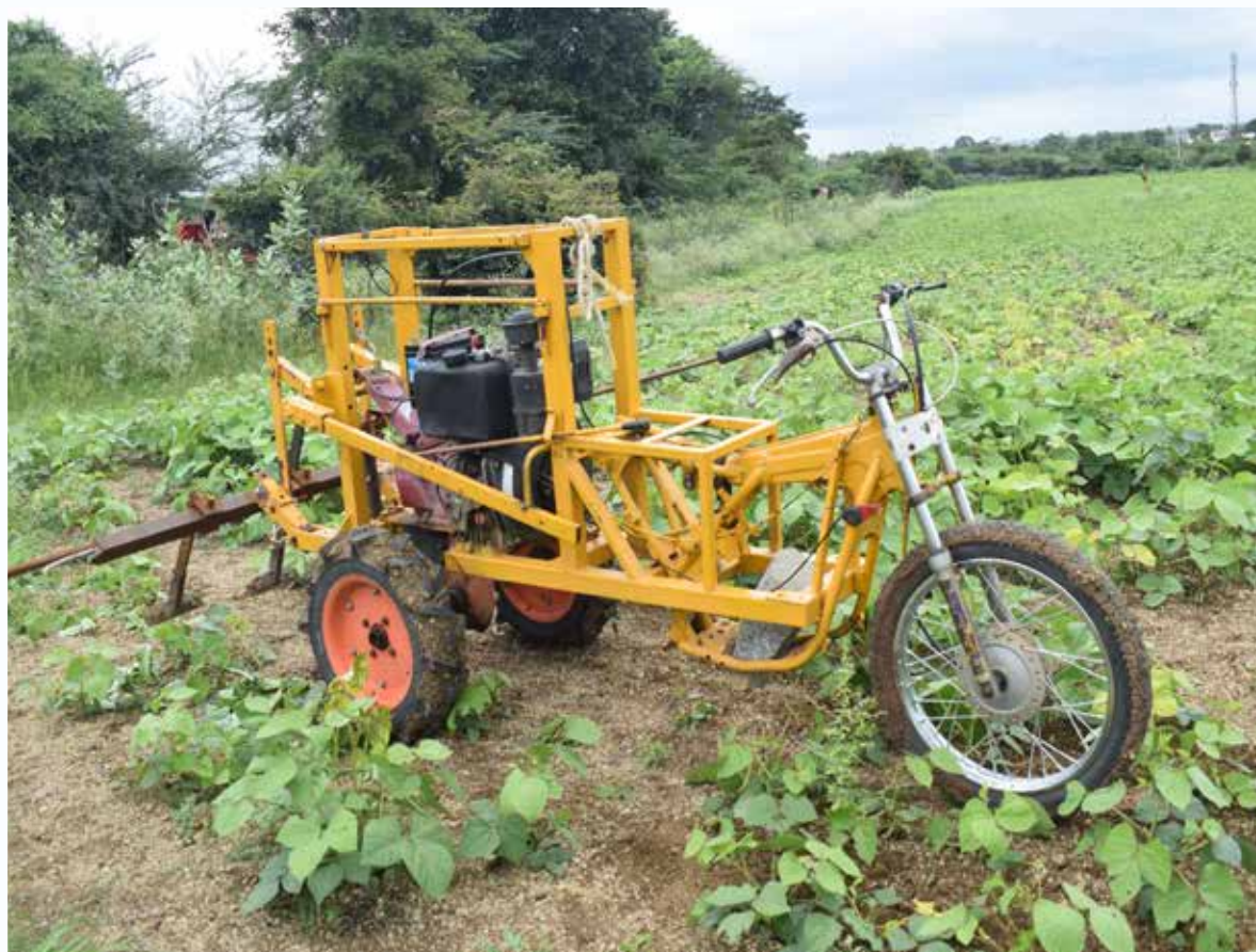
Three wheeler diesel operated machine for spraying and weeding
