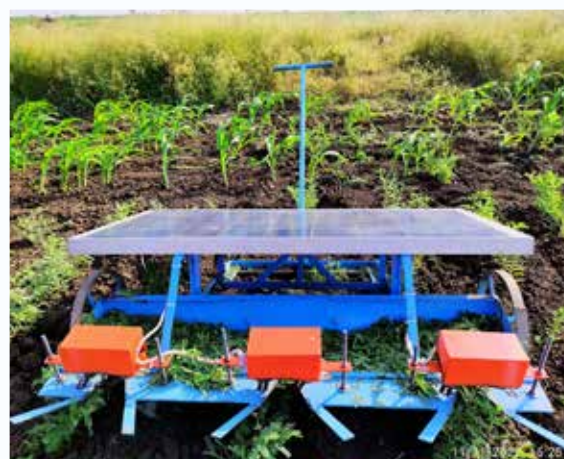
Solar powered plant nipping machine
