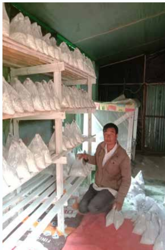
Spawn production in low cost wooden laminar flow cabinet
