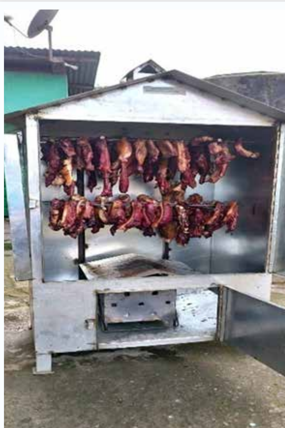
Charcoal-fired multi product drying oven
