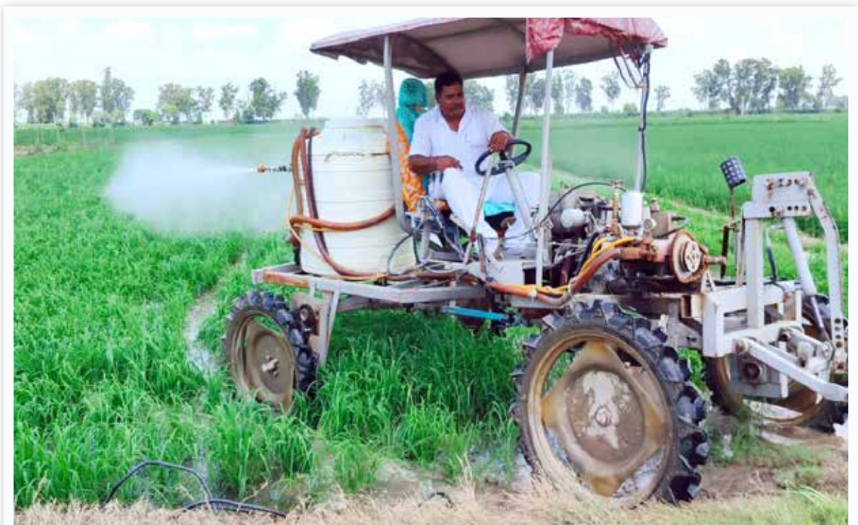
Boom spraying by using multipurpose self made tractor
