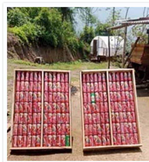
Recycled aluminium cans used in Solar dryer
