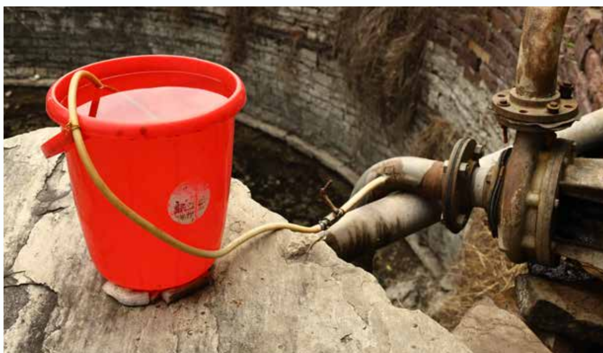
Modified venturi injector for fertigation under low pressure irrigation system
