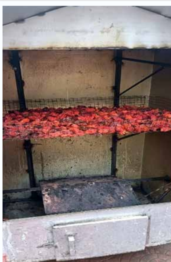
Charcoal-fired multi product drying oven
