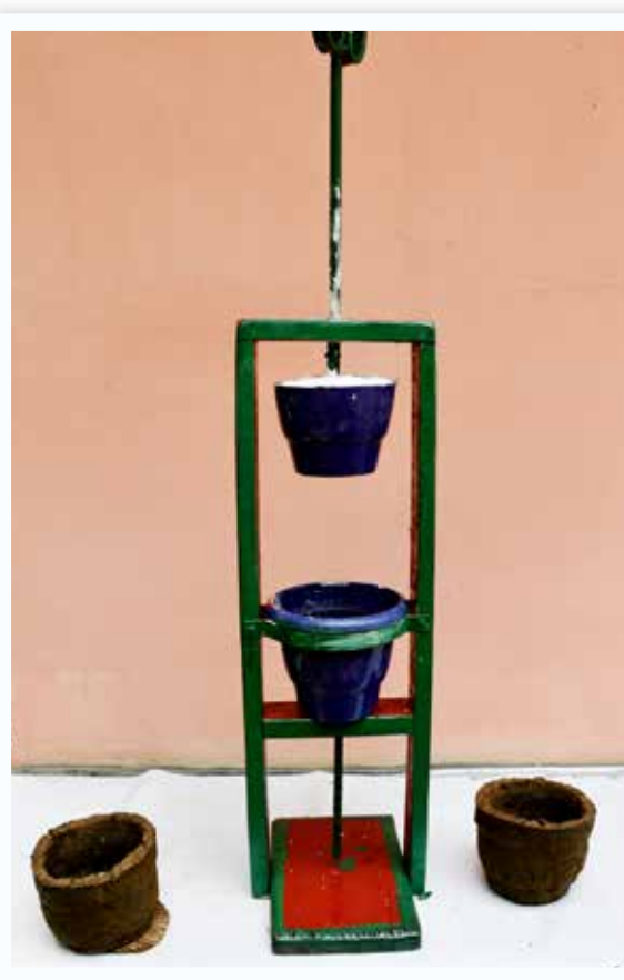
Cow dung pot preparation from Press Machine
