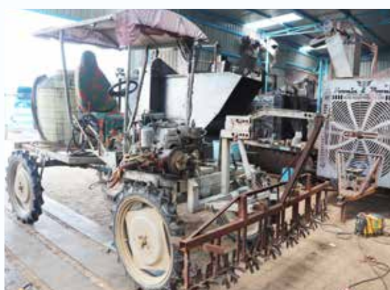
Custom built DSR machine fitted on jugad
