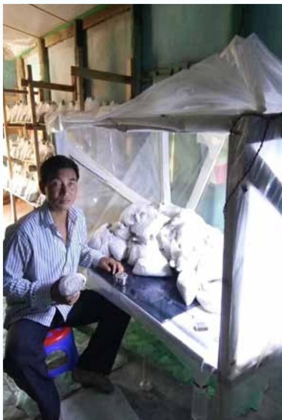
Spawn production in low cost wooden laminar flow cabinet
