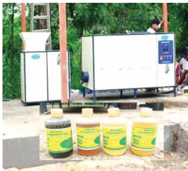
Customized drum type composting unit for enhance decomposition of organic residues.
