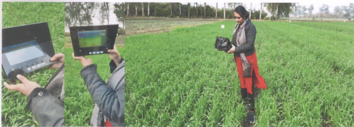
Capturing of wheat image by RGB-Thermal imager
